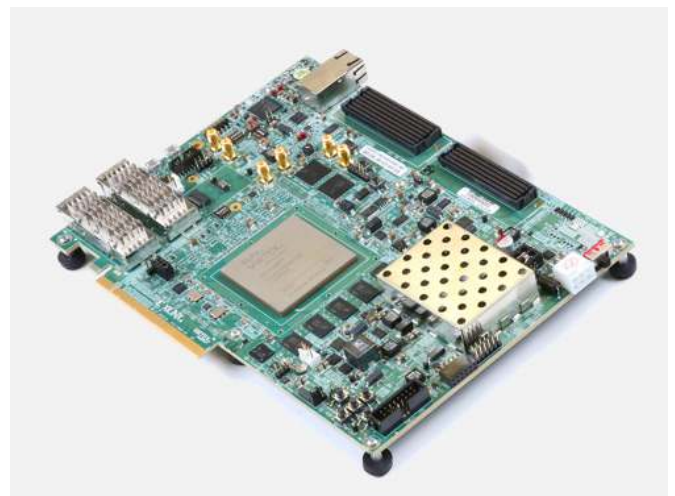
Figure 1. Xilinx VCU118 development board. The VCU118 has a Samtec FireFly™ 4-lane socket and two QSFP28 4-lane sockets.
