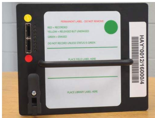
Figure 3: Disk-module labeling and mini-SAS cable connections; color codes must match.
